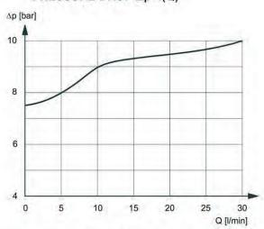
Pressure drop with flow A -> T through the compensator.
