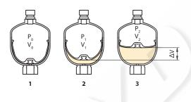
P<sub>0</sub> = (nitrogen precharge pressure) and V<sub>0</sub> = (gas effective volume) correspond to precharge conditions. Hydraulic pressure value is lower than precharge value, i.e. the membrane expansion is maximum and there is no fluid inside
