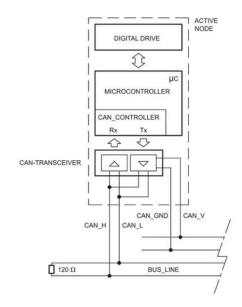
N.B.: insert a 120  $\Omega$  resistance on pin 4 and pin 5 of the CAN connector when the valve is the closure knot of the CAN network.
