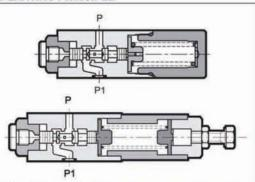
— The MZD valve is a three-way spool type direct operated pressure reducing valve. It is normally open in the rest position and the hydraulic fluid passes freely from the P1 line to the P line.
