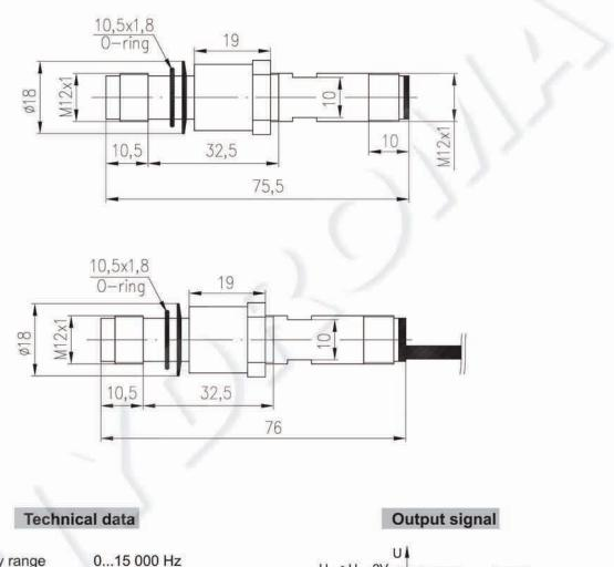
Frequency range0...15 000 HzOutputUniversal PUSH PULLPower supply10-30 VDCCurrent input<20 mA (@24 VDC)</td>Ambient Temperature-40...+125°C [-40...+257°F]ProtectionIP 67Plug connectorM12-SeriesMounting principleISO 6149
