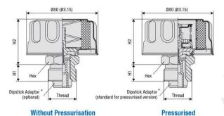
\* Please note: The disptick adaptor is not available for connection threads G1/2 and 1/2 NPT.
