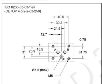
**NOTE**: Port T must never be made. The port P must be made only for RPC1 - \*/CTX. Conversion plates are available.
