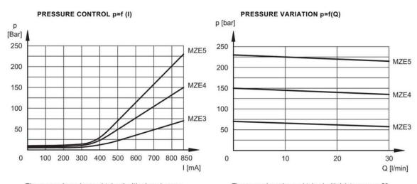
The curves have been obtained with closed users (without flow).
