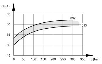
The noise pressure levels were measured in a semianecoic room, at an axial distance of 1 m from the pump.
