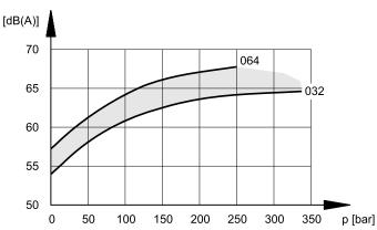
The noise pressure levels were measured in a semi-anecoic room, at an axial distance of 1 m from the pump.
